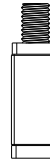
U2 (ADR7278) Fit 7/8 Square Tube Exp. 0.852 - 0.927 1/4 Square Metal Top Square Rubber 1/4 Square Metal Base
